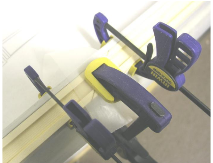
Keep spars flat and straight at splice joint
