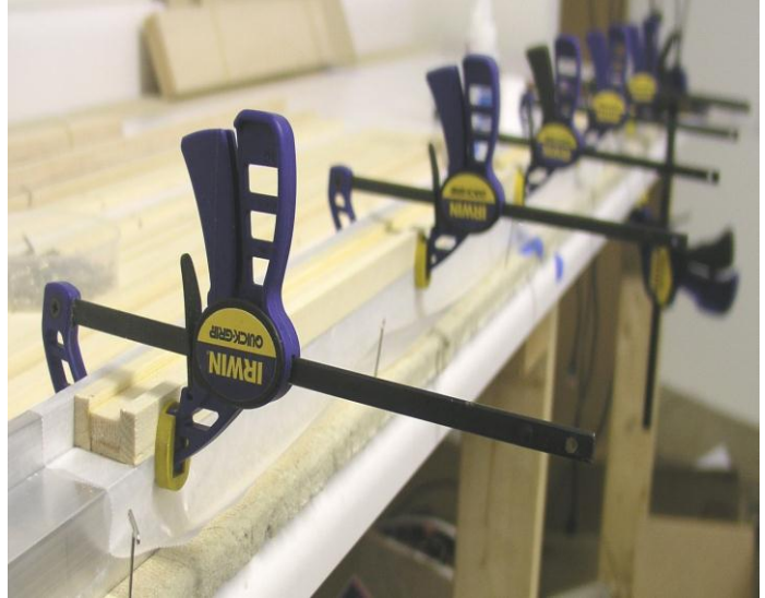
Use support clamps the total length of spar
