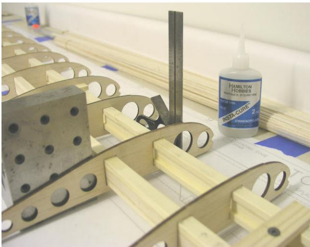
Square ribs to spars, glue in position
