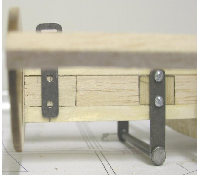
Forward wing skid #315 and fitting #300
