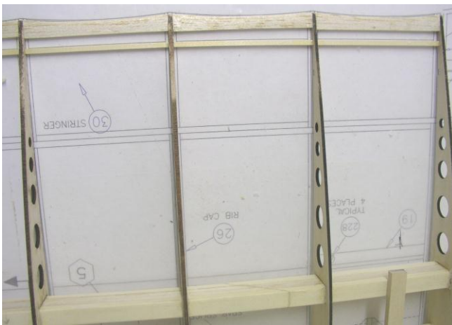
Add trailing edge and stringer to ribs
