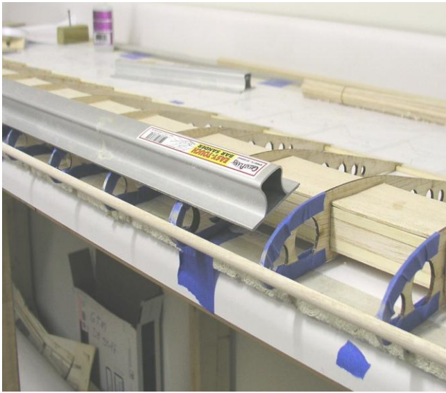
Tape rib noses, sand leading edge to shape
