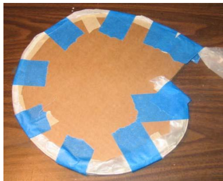
Laminated outline parts taped in place
