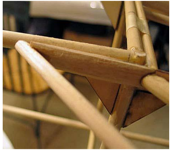
Ensure fwd rib aligns to top longeron
