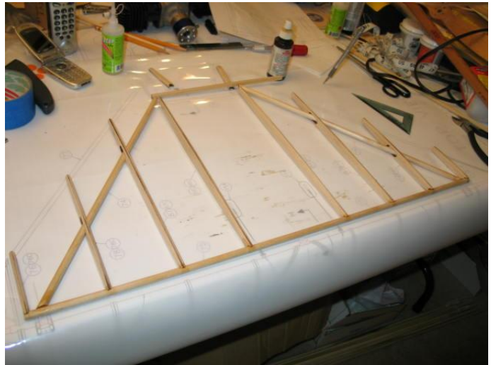
Laminated parts glued into position
