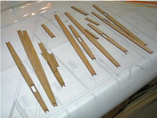
Rib parts ready to be glued together
