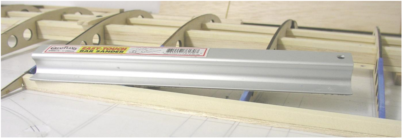
Install trailing edge #50 , tape over ribs, sand trailing edge to shape
