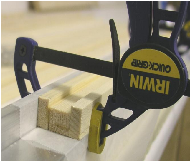
Glue spar pieces together support straight
