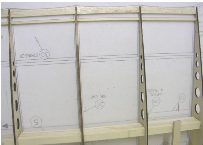
Add trailing edge and stringer to ribs
