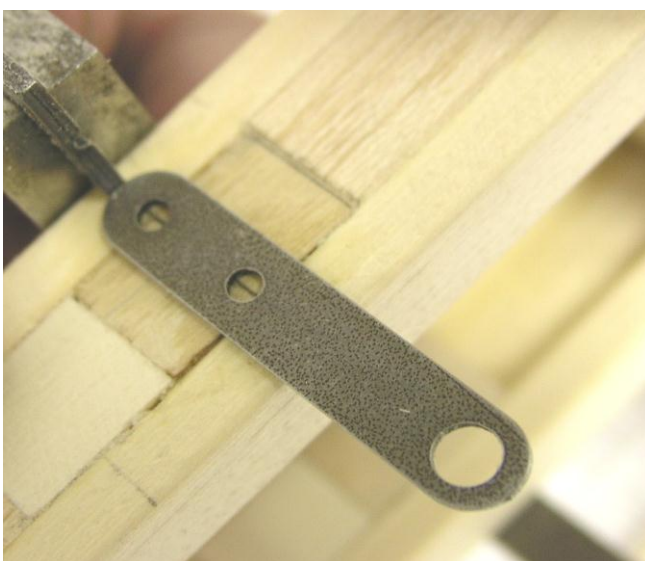
Locate steel interplane fitting #300
