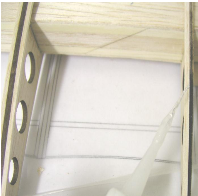
Position and glue rib capping top and bottom
