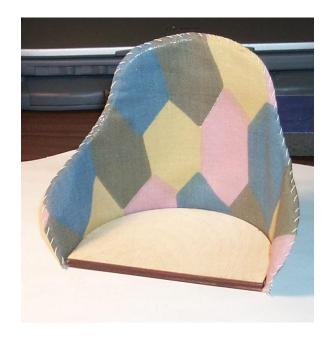
4. Bend the front edges of the aluminum seat #119; this will allow the pilot easy entry and exit. Do not over bend the front edges of the aluminum seat #119; it should have a noticeable slant. Reference the photo below –
