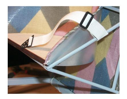
17. Wrap the two 10" rear straps around the rear support **#31**. Carefully, glue the rear strap **#118** back onto itself, **not** gluing it to the support **#31**. See photo below –
