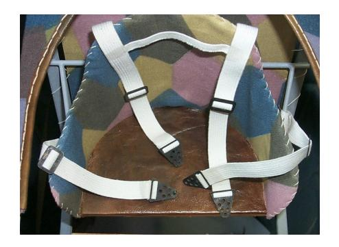
19. All the seat belt plates will mount together. You can tie the hair pin #10 to some left over chord #88 and then secure the hair pin #10 over the nail #712.
