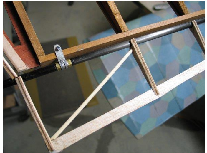
Glue bamboo support #130 in place
