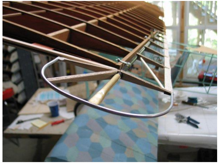
Aileron is ready for covering
