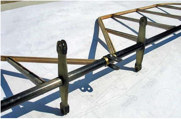
Control horns glued in place
