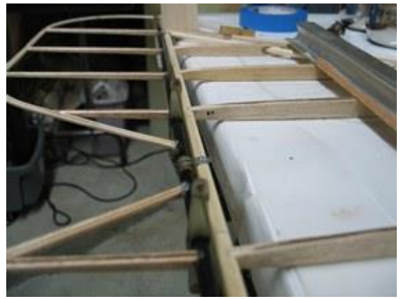
Test fit elevator to stab; fix any warps
