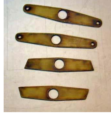
Control horn pieces ready for glue
