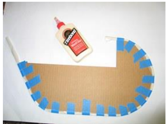
Laminated outline parts taped in place
