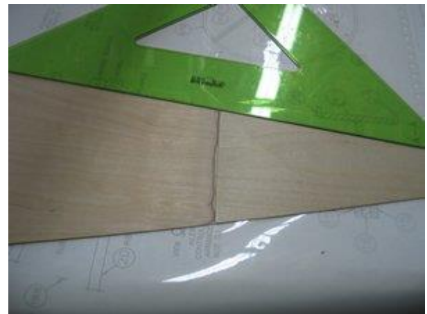
Join halves; should be flat and smooth
