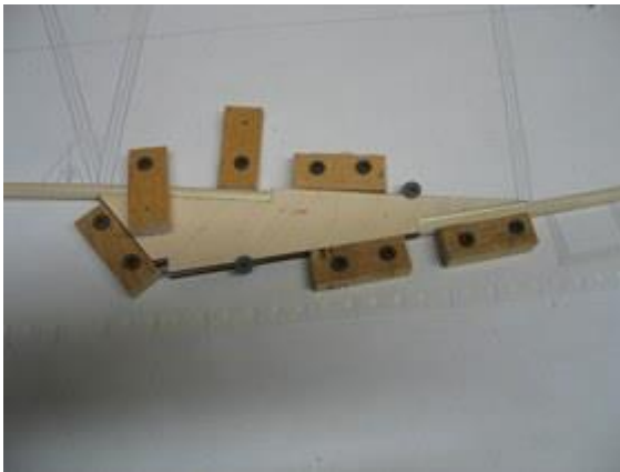
Secure bottom wing joint plywood down
