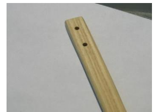
Drill two 1/8" holes
