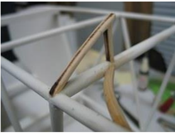
Glue forward arch in position
