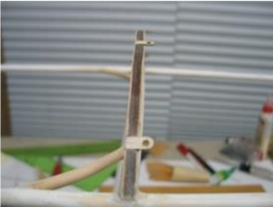
Glue tabs onto rear cockpit arch
