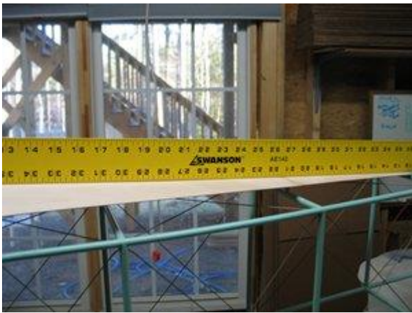
Support turtle deck with scrap wood; Scrap wood goes on top of horizontal Supports.
