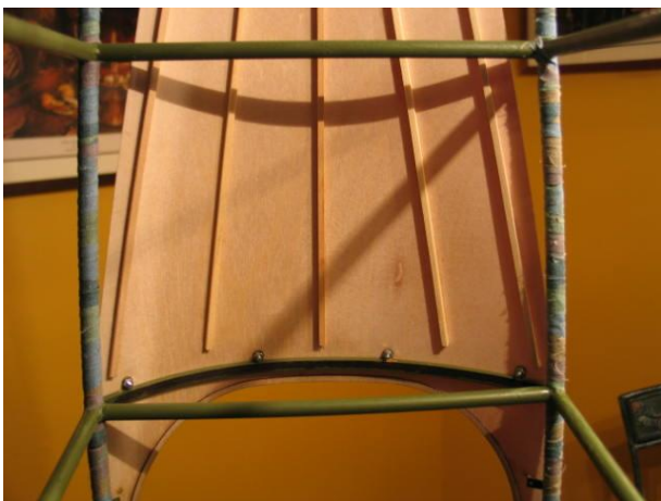
Completed turtle deck underside
