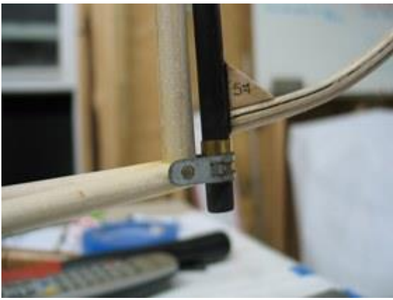
Mount rudder locate hinge holes
