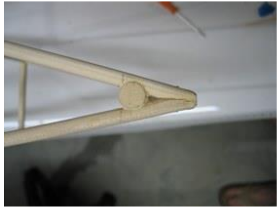
Tail skid and longeron setup
