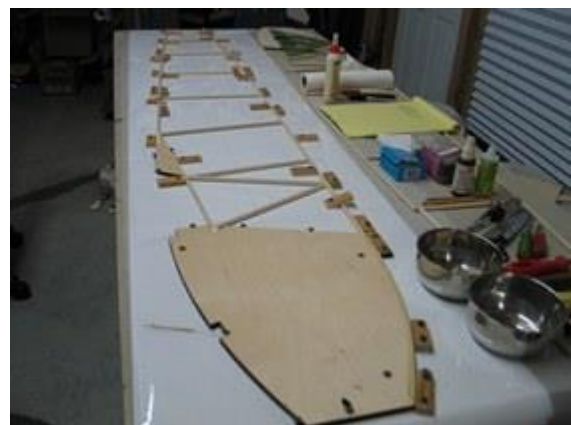
Make a right and left fuselage side
