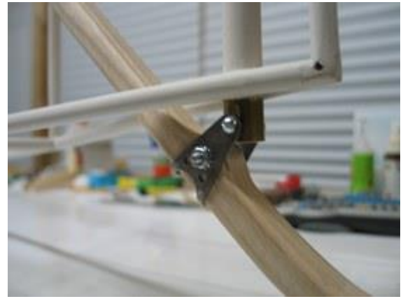
Add brass tube over tail post Drill 7/64 hole; add tail skid
