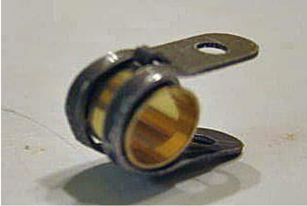
Hinge on center brass bushing
