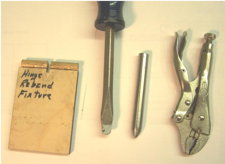
Tools used for hinge bending
