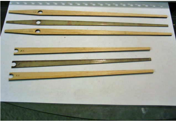
Rib parts ready to be glued together
