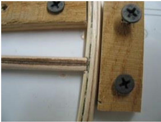
Rudder rib joined in place
