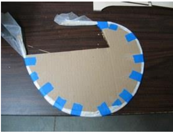
Laminate parts taped in place
