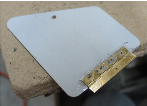
Carefully glue hinge to door first
