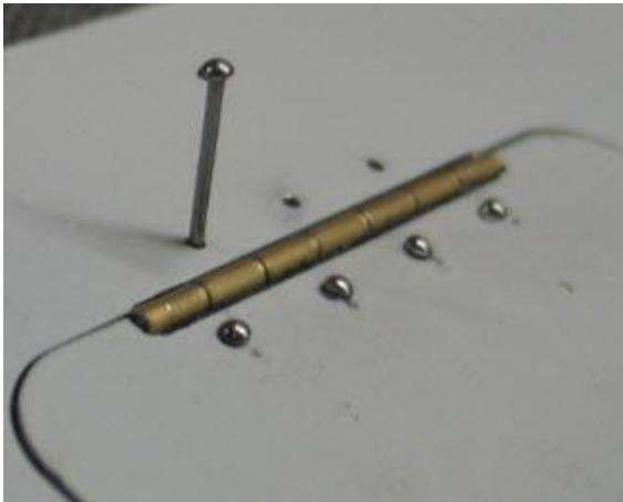
Drill and insert nails into panel
