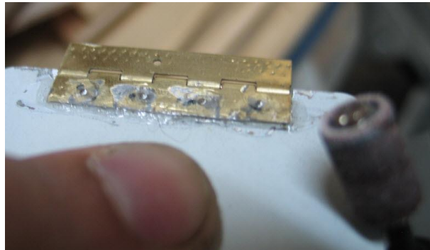
Cut and trim nails almost flush with hinge
