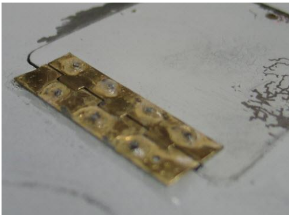
Trim nails almost flush with hinge
