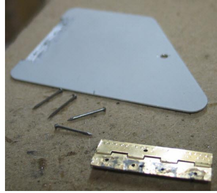
Cut a hinge to fit door notch
