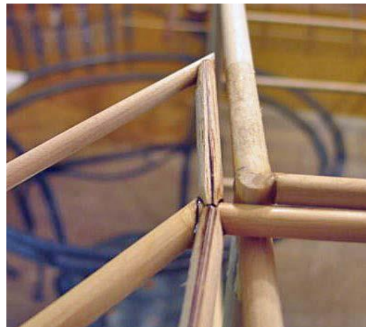
Test fit stab on fuselage; locate fwd rib
