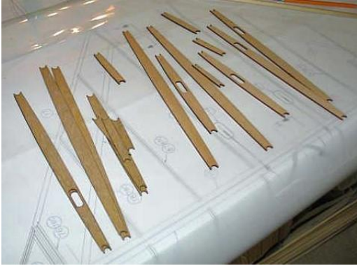
Rib parts ready to be glued together
