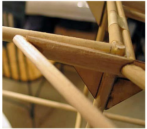
Ensure fwd rib aligns to top longeron
