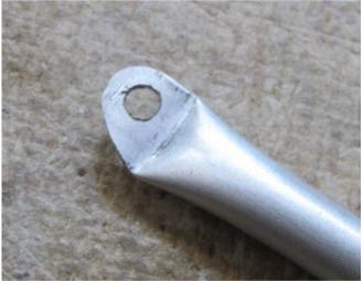
Test fit the tube in place using the plastic screw 3.114. Make any adjustments that are needed. The tube should be straight and not crooked to the gun. Remember the ammo box fitting will be positioned pretty close to the base plate. Note - the screw head should be on the starboard side of the gun when permanently installed. See photo below -
