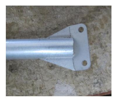
This tube mounts to the top port side longeron 5.3 then goes up to the Vickers forward gun mount. The aluminum tube will be on the outside of the gun mount. Put some scrap 1/8-inch thick wood between the gun muzzle and gas tank which will raise the gun slightly above the gas tank. Test fit this tube in place. Adjust the base plate so the tube goes against the gun mount. See photos below -
