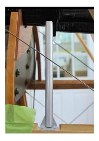
Using a pencil mark the tube where the bottom of the gun mount ends. You will flatten the tube from this line up. See photo below -
