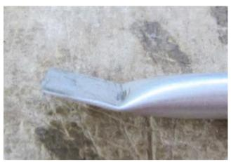
Hold the tube against the gun mount; use a marker to locate the drill hole location. Drill a 5/32-inch hole in the flat tab for screw 3.114 where you made that mark. Carefully, trim and sand the extra part of the tab. See photos below -
