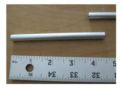
Cut a 2-inch long piece of dowel 5.49. This dowel will require some sanding so it can fit inside the above tube. You can put the dowel in your drill press sanding it. After you sand the dowel cut a 5/8-inch long piece gluing that inside the tube with wood glue. The dowel edge should be flush with the tube edge. See photos below -
