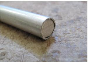
Metal base plate 4.104 will go into this tube end with the dowel. The base plate needs to be bent prior to permanent installation. You can pencil a line on the base plate showing the bend area. Using a vice or something similar slightly bend the base plate. Try to keep the bend crisp and straight. The actual bend angle will be determined when you install the tubing. See photos below -
