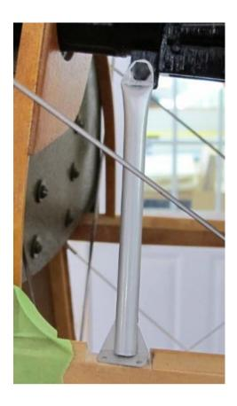
Use two screws 6.78 to secure the base to the top longeron. The edge of the metal base should not extend pass the edge of the top longeron. See photo below -
