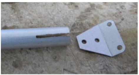
Test fit the base plate into the slot. Using wood glue or similar secure the base plate into the slot keeping the bend straight against the tube as well as the base plate centered in the tube. See photo below -
