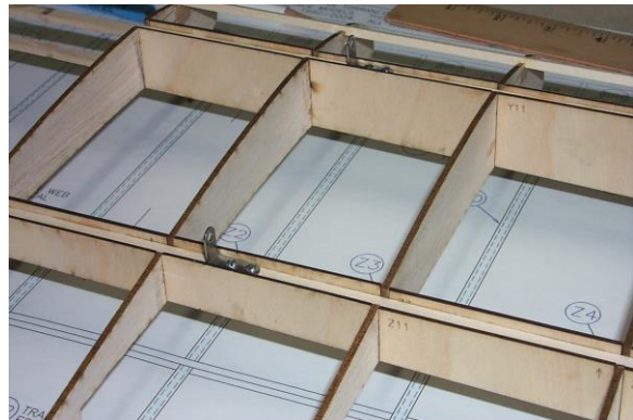
Install n-struts #123 in position, top side
