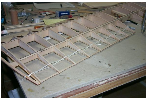
Add rib capping #20 and tape bracing #51
