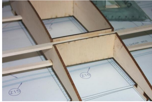
Glue rear spar webbing work outwards
