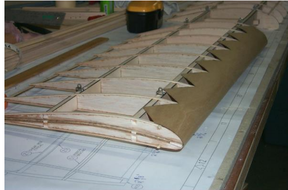
Repeat process for other saw-tooth
