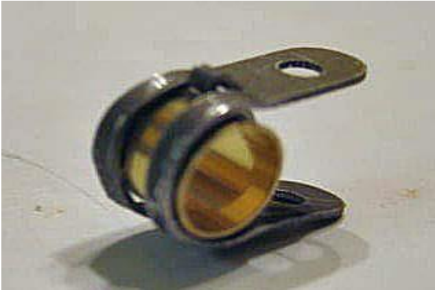
Hinge on center brass bushing
