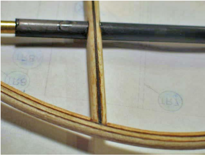
Rudder rib joined in place
