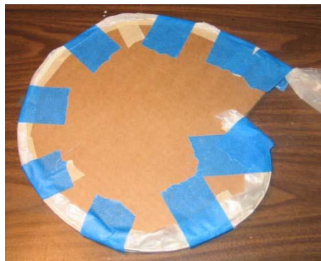
Laminated outline parts taped in place
