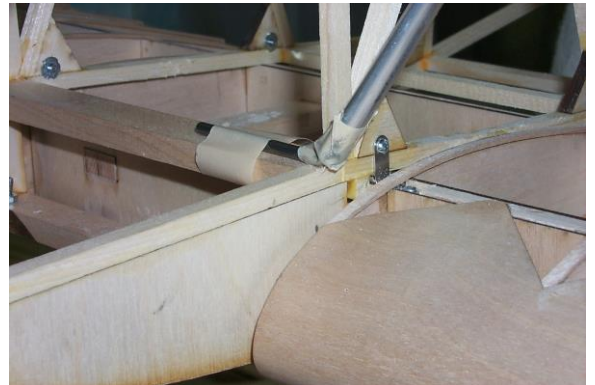
JB Weld, tape music wire, rear strut in place
