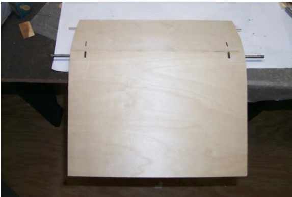
Wrap plywood sheeting around subwing
