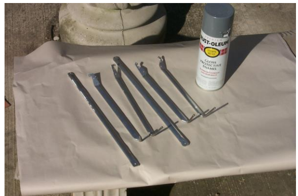
Paint all struts with Rust-O-luem
