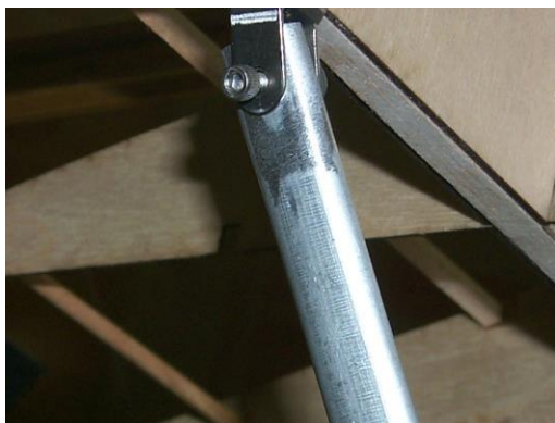
Drill 9/64" holes in struts for top wing
