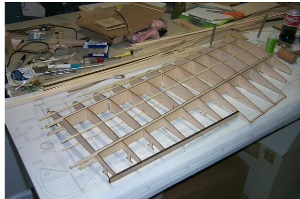
Trim (cut-off) spars passing wing tip
