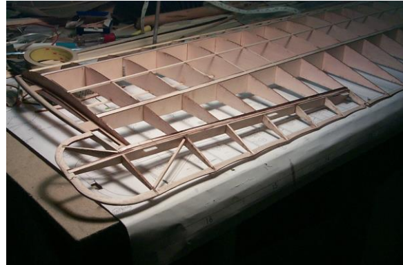
Install and temporarily hinge aileron in place
