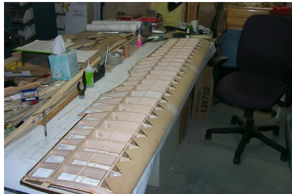
Top wing ready for fabric and servos
