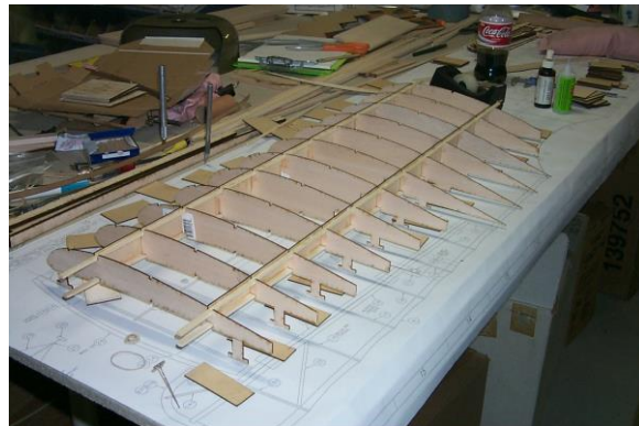
Position and glue rear spar webbing
