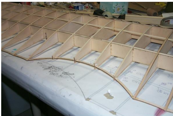
Join wing halves, add balsa #9,10,11
