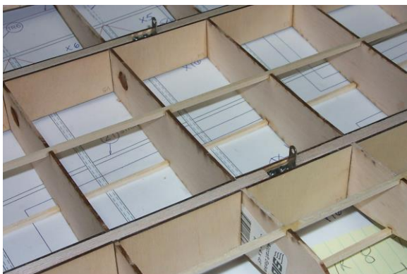
Install n-strut fittings #123 underside
