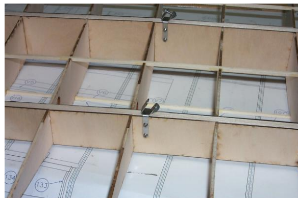
Install wing strut fittings #204
