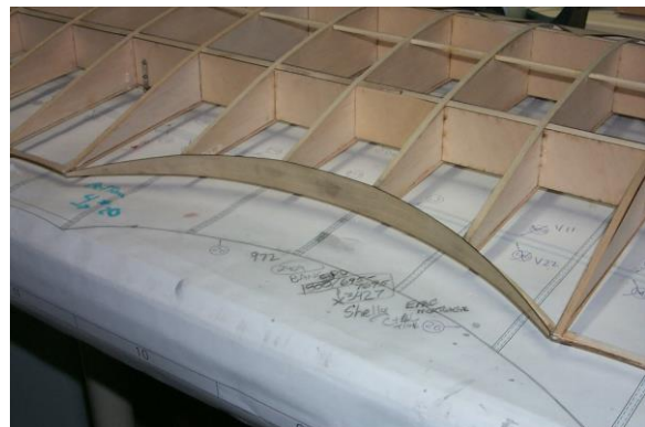
Position and glue cutout plywood #26
