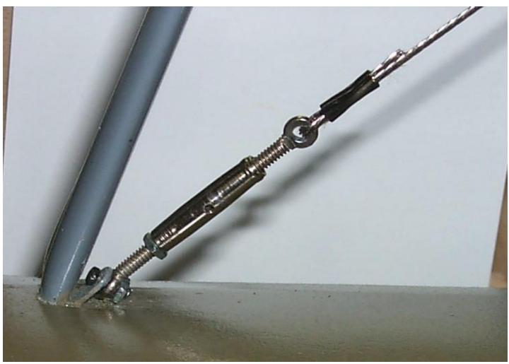
6. Unscrew the turnbuckle #709 so it is loose. Slide another sleeve #720 onto the cable #708. Wrap the cable #708 around the top of strut #307 and back into the newly added sleeve #720. Reference the plans sheet 1 front view. Pull cable #708 tight and crimp sleeve #720. See photo below —
