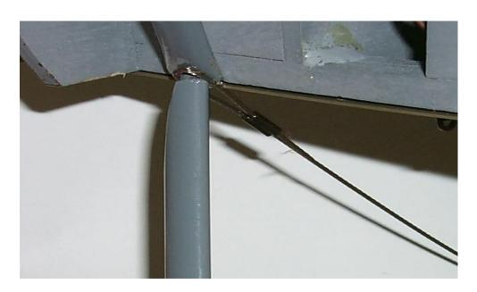
7. Adjust the turnbuckle #709 so the cable #708 tension is tight. The preferred way to use the safety wire #38 to safety turnbuckles #709 is a double wrap (spiral). The turnbuckle #709 has a hex nut on one end, so the double wrap will be changed to a single wrap (spiral). See diagram below -
