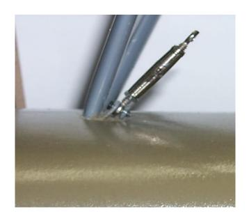
5. Cut two 20" pieces of cable #708. Using small needle nose pliers bend the cable 1" from one end. Pass the cable #708 thru the cable end of the turnbuckle #709; add sleeve #720 and crimp. See photos below –
