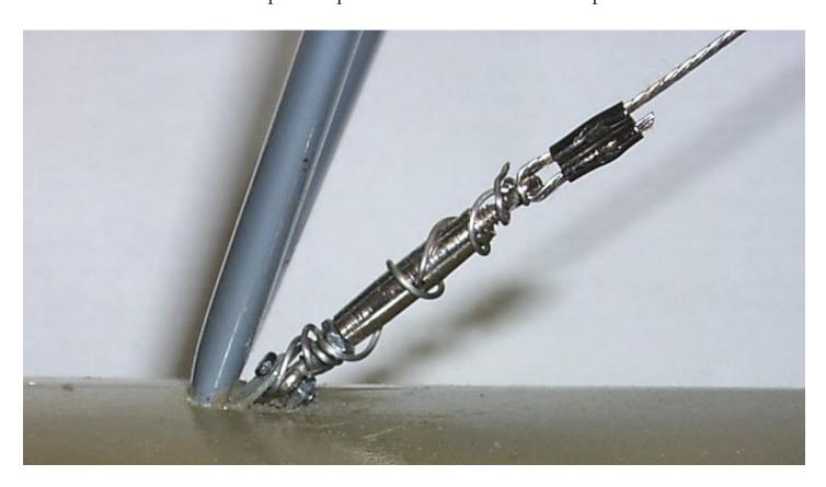
9. This completes the landing gear cabling. Prior to flying inspect the cable tension.
