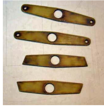
Control horn pieces ready for glue
