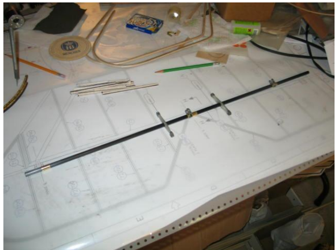
Brass tube, hinges, ctrl horns on carbon tube
