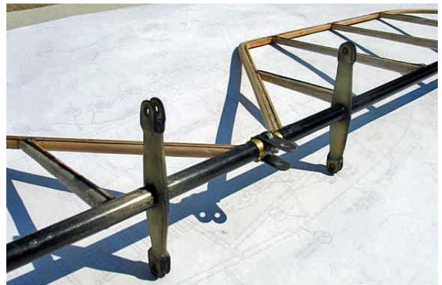
Control horns glued in place
