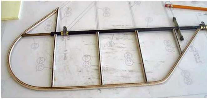
Outline glued in position, ctrl horn is next
