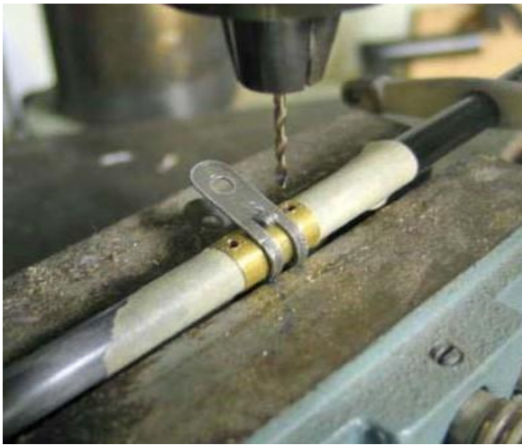
Brass collars being drilled
