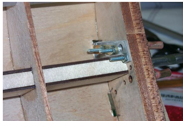
Cut slots in plywood covering for struts
