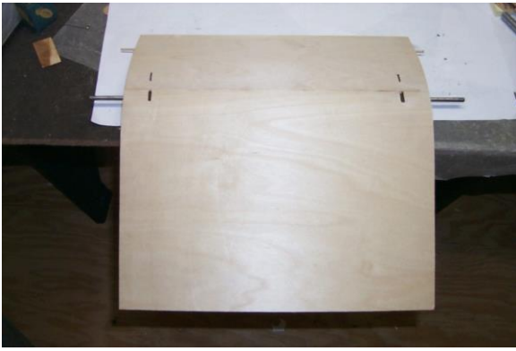
Wrap plywood sheeting around subwing
