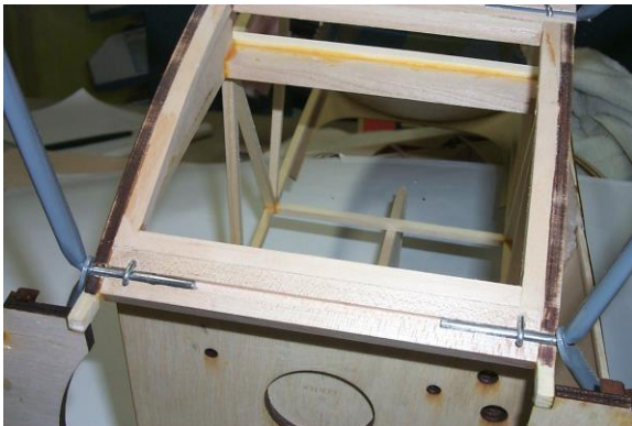
Mount landing gear with j-bolts #306
