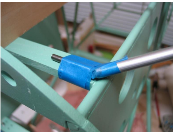
JB Weld to music wire to strut
