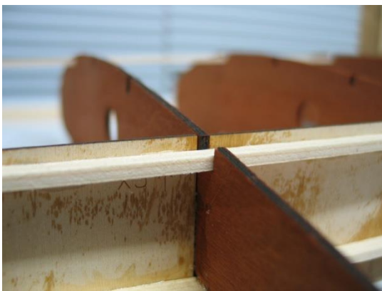
Ensure spar webbing has no gaps
