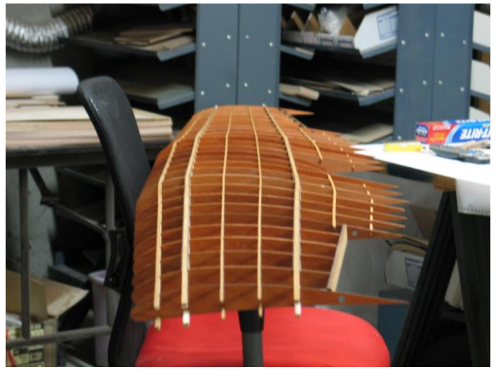
Remove and cover aileron with plywood
