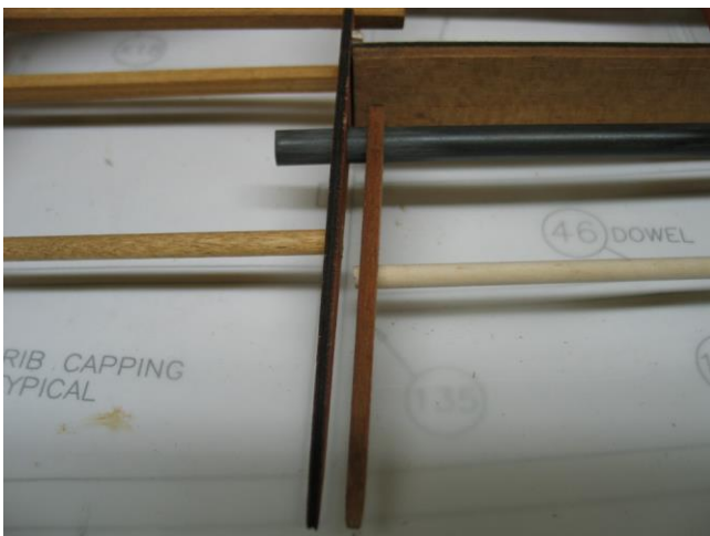
Ensure aileron / wing gap is correct
